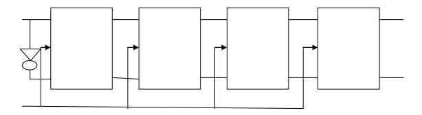
In serial in serial out shift register the binary data is accepted serially i.e one bit at a time is accepted on a line .The stored information is also produced at the output in serial form
